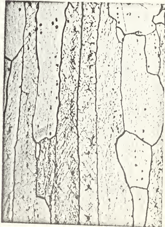
FIG. 24 AT 540°C, UNDER .6%/HR. STRAIN RATE, FOR 3 HOURS (ROCKWELL 30T 42.1)
